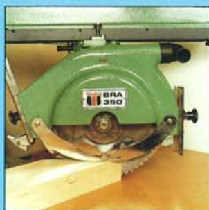
Accurate ripping – universal model only.
