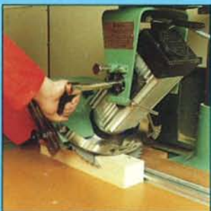
Mitre cross cutting – universal model only.
