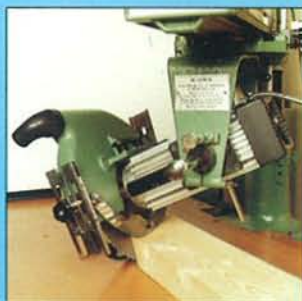
Compound angle cutting – universal model only.
